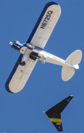
Flight tests have resumed on subscale aircraft that could one day observe the Martian atmosphere and a variant that will improve collection of Earth's weather data. The March flights included two slightly different Prandtl-M aerodynamic models that were air launched from a remotely piloted Carbon Cub. The research validated the airframe that will be the basis for a potential Mars aircraft and the Weather Hazard Alert and Awareness Technology Radiation Radiosonde (WHAATRR) Glider on Earth.
